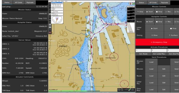
(b) The control terminal in the RCC is based on OpenCPN with a sidebar extension to transfer direct commands and mission maps to the vehicle's GNC.
