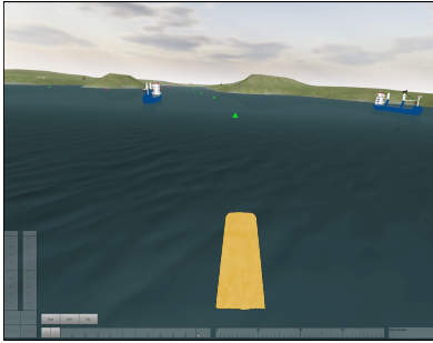
(a) Bridge Command with an XLUUV model of MUM provides the interface between simulated driving physics, the environment, vessel traffic, and the actual testbed.
