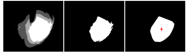
Figure 4: Arc centroid determination; intensity depth reduction, threshold, convex hull and centroid determination from left to right
