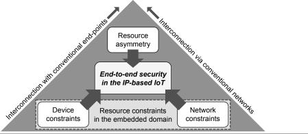
**Figure 1.1** Main factors that challenge the design adequacy of standard end-to-end IP security protocols in the context of networked embedded devices and the IP-based IoT.
