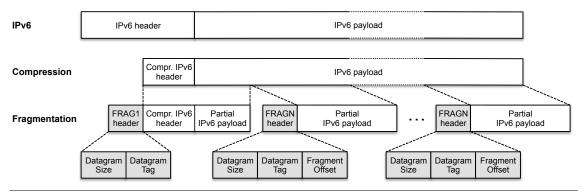
**Figure 2.8** The packet structure before (top) and after (bottom) after the 6LoWPAN header compression and packet fragmentation mechanisms were applied to an IPv6 packet. The additional 6LoWPAN fragmentation headers are marked in gray. Notably, only the first 6LoWPAN fragment (i.e., the FRAG1) contains routable IPv6 header information.
