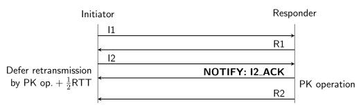
**Figure 4.15** The Responder indicates its anticipated I2 message processing time in the I2\_ACK parameter of our newly introduced intermediate NOTIFY message. When receiving this reception acknowledgement, the Initiator adapts its retransmission timeout to the indicated I2 processing time plus half the worst-case anticipated RTT for the transmission of the R2.
