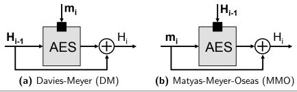
**Figure 6.12** One-way compression functions. The DM and MMO modes of operation afford the use of the AES block cipher to build a hash function via the Merkle-Damgård construction.
