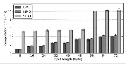
**Figure 6.19** Computation overhead for the generation or the verification of a single content token. The bars represent the average over 100 measurement runs for each input size. The error bars illustrate the observed the standard deviation. Both AES-based hash functions consistently outperform SHA-1. Moreover, the DM-based and MMO-based hash functions only exhibit a modest performance difference.
