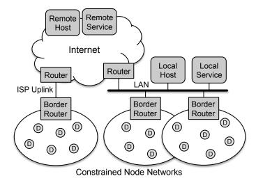
**Figure 2.4** The network scenario in scope of our work. IP-enabled constrained devices (D) form constrained node networks. Border routers connect these networks, e.g., to a local area network or to the Internet. The connectivity affords communication between constrained devices from separate network domains and enables the interconnection with local/remote hosts or services.
