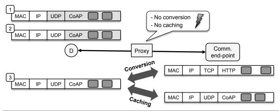
**Figure 7.2** The network-layer and transport-layer protection of standard end-to-end IP security (marked in light gray for 1 and 2, respectively) prevent cross-protocol conversion middleboxes or caching proxies from operating on traversing network packets. In contrast, selective end-to-end payload security (3) only encrypts confidential and integrity-protects immutable application data (marked in dark gray) and, thus, affords provisioning of these on-path middlebox functions.
