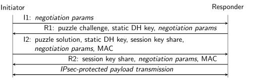
**Figure 3.7** Sequence diagram of the HIP DEX handshake. Cipher suite negotiation, peer authentication, and key agreement are performed in a four-way message exchange.
