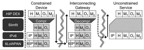
**Figure 4.28** Integration of the Slimfit compression layer with an existing network stack. Arrows indicate the processing flow for a HIP DEX message with an interconnecting gateway. Slimfit compresses the HIP header (H), reorders mandatory  $(M_i)$  and optional  $(O_j)$  parameters, and compresses or elides these parameters. The dashed arrow indicates that the HIP DEX message skips the Slimfit and the 6LoWPAN adaptation layers for message transmission.
