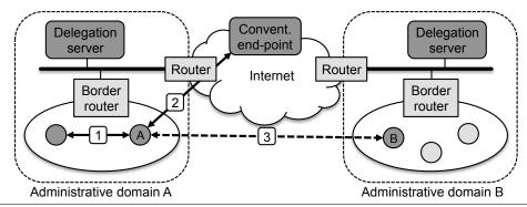
**Figure 7.1** The presented handshake delegation architecture provides a framework for intradomain authorizations between networked embedded devices (1) and inter-domain authorizations with conventional communication end-points (2). Authorizations involving memory-constrained embedded devices from remote administrative domains (3) are future work.
