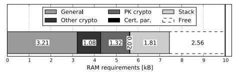
**Figure 5.1** RAM requirements of a protocol implementation with support for the certificate-based DTLS handshake. Constrained devices with similar memory limitations as the TelosB platform (i.e., 10 kB of RAM as indicated by the bold vertical line) only have 2.56 kB of RAM available for the underlying operating system and the actual application logic.
