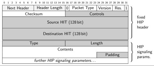
**Figure 4.25** The HIP message structure consists of a fixed protocol header and a number of HIP signaling parameters. Each signaling parameter has a type-length-value encoding and includes individual parameter padding. Compressible information is marked gray. The fields marked light gray can be handled by existing compression mechanisms at the 6LoWPAN layer.
