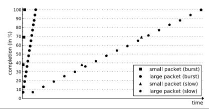
**Figure 6.15** Packet score at a reassembling node based on the percentage of completion. Fragmented packets, which are sent in short bursts, quickly gain a high packet score. In contrast, fragmented packets, which are transmitted at a low sending rate and reserve the reassembly resources for extended periods of time, only slowly increase the packet score.
