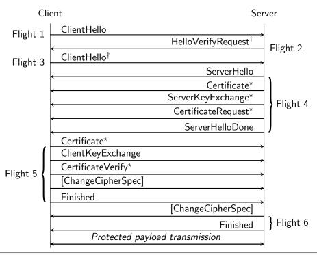
**Figure 3.6** Sequence diagram of the DTLS handshake. Messages marked with a dagger ( $^{\dagger}$ ) implement a return-routability test for DoS protection purposes. Starred messages ( $^{\star}$ ) are optional and are only required depending on the negotiated cryptographic primitives.
