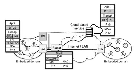
**Figure 1.2** IoT network scenario consisting of networked embedded devices (D), interconnecting gateways (GW) and a cloud-based service. The layers in the network stack that are affected or newly introduced by our contributions are marked in gray. The arrows represent communication paths via local network infrastructure and potentially the global Internet. The dashed lines indicates handshake delegation via the newly introduced delegation server (DS).
