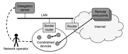
**Figure 5.3** The handshake delegation architecture consists of the following entities (marked in dark gray): a network operator, a delegation server, constrained devices, and remote communication end-points. Continuous arrows highlight the different connections that are supported by the presented architecture. Dashed arrows indicate responsibilities of the network operator.
