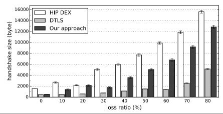
**Figure 4.22** Transmission overhead of the standard *HIP DEX*, the *DTLS*-based, and our adaptive retransmission strategy for different loss probabilities. The error bars depict the 99% confidence intervals. The DTLS-based strategy causes the lowest transmission overhead, while *our approach* outperforms standard HIP DEX.
