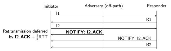
**Figure 4.18** Spoofed I2 reception acknowledgments would enable an eavesdropping adversary to arbitrarily delay the protocol handshake. Importantly, the adversary cannot force the Initiator into setting the I2 retransmission timeout below half the worst-case anticipated RTT.
