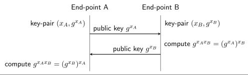
**Figure 3.2** The DH key exchange. Both communication end-points A and B derive the same secret key  $g^{x_Ax_B}$ . However, only public information  $g^{x_i}$  is revealed on the communication path.
