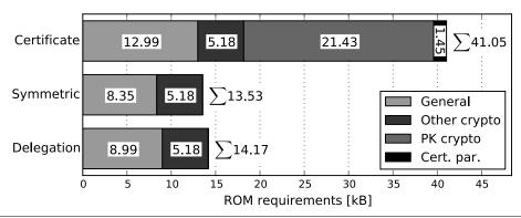
**Figure 5.12** ROM requirements of the DTLS implementation variants supporting the certificate-based handshake, the symmetric-key-based handshake, and the handshake delegation architecture. The public-key-related protocol functionality constitutes the major contributor to the ROM requirements of the certificate-based DTLS handshake. Handshake delegation and the symmetric-key-based handshake exhibit similar ROM requirements.
