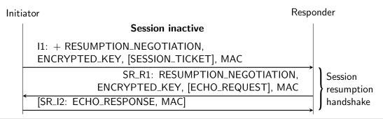
Figure 4.3 The abbreviated session resumption handshake for HIP DEX. Brackets denote optional messages and parameters that depend on the actual session resumption type.
