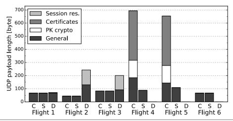
**Figure 5.15** Transmission overhead of the certificate-based DTLS handshake (C), the symmetric-key-based DTLS handshake (S) and the presented handshake delegation procedure (D) aggregated on a per-flight basis. The handshake delegation procedure causes a reduced transmission overhead compared to the certificate-based DTLS handshake and a similar transmission overhead as the symmetric-key-based DTLS handshake.
