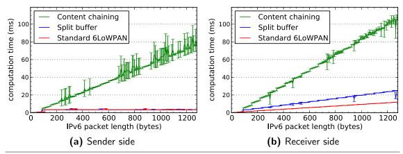
**Figure 6.20** Processing time at the 6LoWPAN layer for the standard 6LoWPAN fragmentation mechanism, the content-chaining scheme, and the split buffer approach. The error bars denote the standard deviation. The split buffer approach only causes a modest overhead, whereas the content-chaining scheme incurs a noticeable overhead at the sender and at the receiver.
