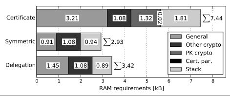
**Figure 5.11** RAM requirements of the DTLS implementation variants supporting the certificate-based handshake, the symmetric-key-based handshake, and the handshake delegation procedure. Handshake delegation requires slightly more RAM resources than the symmetric-key-based handshake, but considerably less than the certificate-based handshake.
