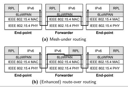
**Figure 6.7** The packet processing path inside a constrained node network that employs mesh-under routing or (enhanced) route-over routing. While forwarding nodes can remain oblivious to the 6LoWPAN packet fragmentation in case of mesh-under routing, these node are required to act on 6LoWPAN-fragmented IPv6 packets in case of (enhanced) route-over routing.
