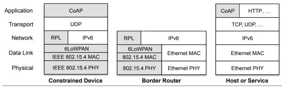
**Figure 2.6** Comparison of the IP network stacks for constrained devices, border routers, and conventional hosts or services. Protocols that are specifically designed for the IP-based IoT are marked in gray. Notably, the IPv6 adaptation layer 6LoWPAN and the RPL routing protocol are only deployed on constrained devices and border routers, whereas the application protocol CoAP should also be supported by conventional hosts and services.
