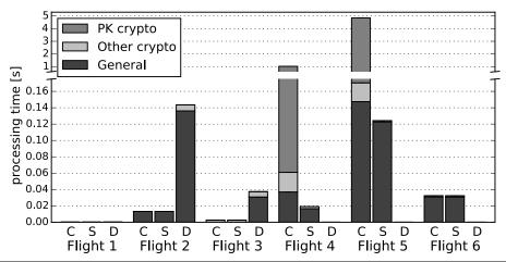
**Figure 5.14** Server-side computation overhead of the certificate-based DTLS handshake (C), the symmetric-key-based DTLS handshake (S) and the handshake delegation procedure (D) aggregated on a per-flight basis. The overheads at the server are similar to those at the client.
