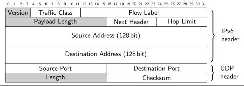
**Figure 2.7** IPv6 and UDP header structure. Header fields that always are compressible are marked in gray. All other fields are only compressible depending on upper or lower layer header information or require the header field to contain specific values for compression purposes.
