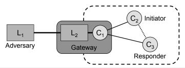
**Figure 4.21** Evaluation setup for our collaborative puzzle-based DoS protection mechanism. Supported by the on-path gateway ( $C_1$  and  $L_2$ ), the Responder ( $C_3$ ) was able to protect itself against an unconstrained adversary ( $L_1$ ). At the same time, the benign Initiator ( $C_2$ ) could still perform a limited amount of legitimate handshakes with the Responder ( $C_3$ ).
