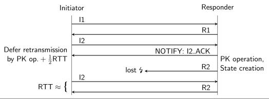
**Figure 4.16** Repeated R2 retransmissions no longer involve computationally expensive public-key operations. Instead, the Responder can immediately reply to the retransmission-triggering I2 message based on its previously established session state. Consequently, the Responder does not send another NOTIFY message in case of an R2 retransmission. Moreover, following a NOTIFY, the Initiator sets the I2 retransmission timeout to the worst-case anticipated RTT.
