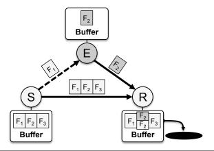
**Figure 6.4** The fragment duplication attack. Eve (E) overhears 6LoWPAN fragments from the legitimate sender (S) and injects a spoofed fragment with altered fragment content. Due to overlapping fragment content, the recipient (R) drops the entire IPv6 packet.
