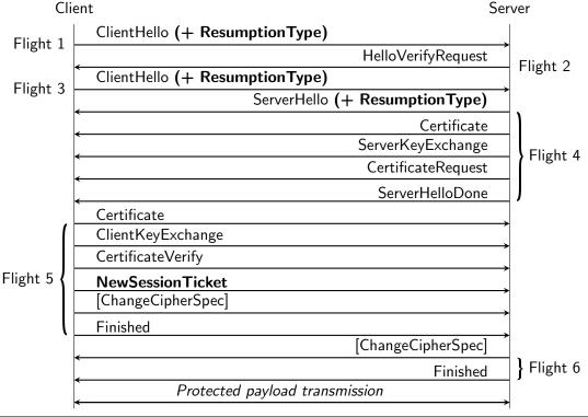
**Figure 4.4** Session resumption type negotiation and client-side state-offloading during the initial connection establishment handshake of the DTLS protocol. Session resumption-related information is marked bold. Brackets denote DTLS protocol extensions.
