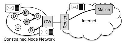
**Figure 6.3** The attacker model for our security analysis of the 6LoWPAN fragmentation mechanism. The adversaries Eve (E) and Mallory (M) are co-located with constrained devices (D) inside a constrained node network. Malice is situated outside the target network. Arrows indicate specific packet forwarding paths. The dashed line represents overhearing.
