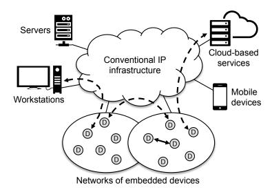
**Figure 2.1** Abstract IoT network scenario consisting of networked embedded devices (D) and conventional communication end-points such as workstations and servers. Arrows indicate network traffic flows with a special focus on interactions that involve networked embedded devices. Dashed arrows represent traffic flows that involve conventional IP infrastructure.
