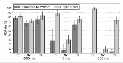
**Figure 6.17** Successful reception of legitimate UDP packets (1280 byte) at the application layer of the target device during the buffer reservation attack. The split buffer approach consistently outperforms the unmodified 6LoWPAN fragmentation mechanism of the Contiki OS independent from the adversary's sending behavior and the sender's transmission offset.
