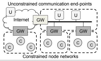
**Figure 4.9** Example network scenario depicting the interconnection of constrained (C) and unconstrained (U) communication end-points in the IoT. Gateways (GW) that interconnect a constrained node network with adjacent network domains are marked in dark gray.
