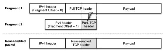
**Figure 6.1** Packet filter evasion based on overlapping fragments. The on-path packet filter inspects the first fragment that appears to be legitimate and applies the same filter decision to the second packet fragment. The second fragment, however, overwrites, e.g., the TCP flags in the header of the transport layer during packet reassembly at the victim host (marked in gray). This effectively conceals the actual TCP flag combination from the packet filter.
