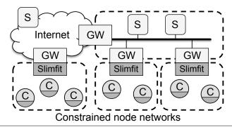
**Figure 4.27** Constrained devices (C) communicate with each other and with local or Internet-based services (S) via a gateway (GW). Only network entities that belong to a constrained node network are equipped with our Slimfit compression layer (marked dark in gray). All other network entities can remain oblivious to the Slimfit-compressed HIP message wire-format.
