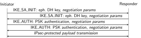
**Figure 3.8** Sequence diagram of the Minimal IKEv2 handshake. The IKE\_AUTH exchange and the IPsec payload channel are protected based on an ephemeral DH key agreement. The peer authentication performed during the IKE\_AUTH exchange is based on Pre-Shared Keys (PSKs).
