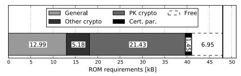
**Figure 5.2** ROM requirements of a DTLS protocol implementation with support for the certificate-based handshake. Only about 6.95 kB of ROM remain for the underlying operating system and the actual application logic in case of a constrained device with similar memory limitations as the TelosB platform (i.e., 48 kB of ROM as indicated by the bold vertical line).
