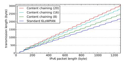
**Figure 6.18** Transmission overhead of the content-chaining scheme for different token and packet sizes (with all headers) compared to the standard 6LoWPAN fragmentation mechanism. The content token size in byte is shown in brackets. Truncated content tokens achieve a significant reduction of the transmission overhead, especially for large fragmented packets.
