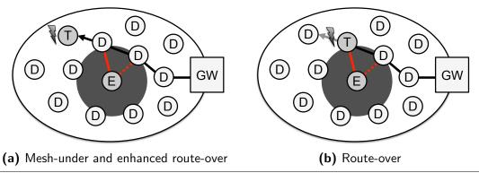
**Figure 6.8** Susceptibility of constrained devices (D) against the identified 6LoWPAN fragmentation attacks depending on the employed fragment forwarding mechanism. Mesh-under and enhanced route-over routing allow Eve (E) to target constrained devices (T) beyond her one-hop neighborhood. With route-over routing, she is limited to her one-hop neighborhood.
