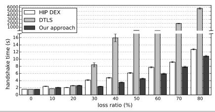
**Figure 4.23** Handshake run-time of the standard *HIP DEX*, the *DTLS*-based, and our adaptive retransmission strategy depending on the loss probability. The error bars depict the 99% confidence intervals. *Our approach* outperforms the other considered retransmission strategies for nearly all loss probabilities.
