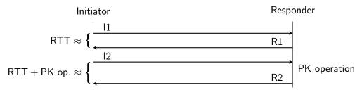
**Figure 4.14** Expected delay between the transmission of the Initiator's and the reception of the Responder's handshake messages depending on the message type. The combined transmission delays of the I2 and the R2 messages along with the I2 processing time at the Responder quickly exceed a purely RTT-based retransmission timeout.
