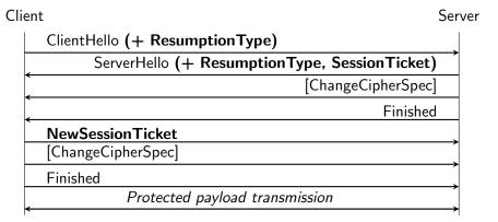
**Figure 4.5** Abbreviated handshake with client-side state-offloading for DTLS. Session resumption-related information is marked bold. Brackets denote DTLS protocol extensions.
