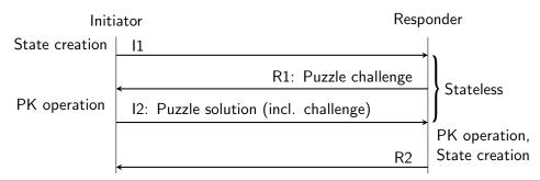
**Figure 4.7** The standard HIP DEX handshake with a specific focus on the expensive protocol operations and the existing DoS protection mechanisms. PK denotes a public-key operation.
