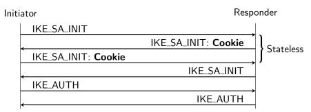
**Figure 4.13** The cookie-based DoS protection mechanism of the original IKEv2 protocol. The Responder includes a cookie notification payload in its IKE\_SA\_INIT response. The Initiator then has to repeat the IKE\_SA\_INIT exchange and echo back the received cookie value.
