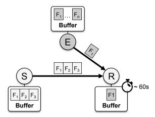
**Figure 6.5** The buffer reservation attack. Eve (E) sends a single 6LoWPAN fragment to the resource-constrained recipient (R). Eve, however, does not complete the partial IPv6 packet with the remaining 6LoWPAN fragments. As a result, the reassembly buffer at the recipient is maliciously occupied until the reassembly timeout expires. During this time, the recipient cannot process other fragmented packets that originate from a legitimate sender (S).
