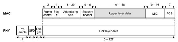
Figure 2.2 IEEE 802.15.4-2003 frame format at the physical and the link layer. The frame space available for upper layer protocol data is marked gray. Size indications are given in byte.
