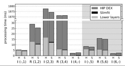
**Figure 4.33** Message processing time for the connection establishment and the connection teardown (marked with a gray background) for the standard HIP DEX protocol (H) and with our Slimfit compression layer (S) for the Initiator (I) and the Responder (R). The numbers in brackets denote processing of the i-th and generation of the (i+1)-th handshake message.
