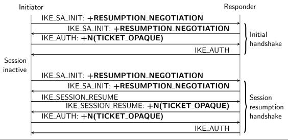
**Figure 4.6** Sequence diagram of the session resumption type negotiation and Initiator-side state-offloading functionalities for Minimal IKEv2.  $N(\cdot)$  denotes an IKEv2 notification payload.
