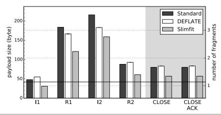
**Figure 4.31** HIP message size for the HIP DEX connection establishment handshake and a subsequent connection teardown exchange (marked with a gray background) for the *standard* HIP DEX protocol, with *DEFLATE* compression, and with our *Slimfit* compression layer. The continuous line indicates the 6LoWPAN fragmentation threshold in our evaluation setup. The dashed lines then indicate the maximum payload size of the individual 6LoWPAN fragments.
