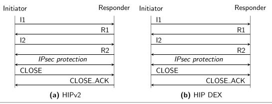
**Figure 4.24** Comparison of the connection establishment handshake and the connection teardown exchange for HIPv2 and HIP DEX. Notably, both protocols employ the same exchange structure. This is because HIP DEX inherits the primary message exchanges from HIPv2.
