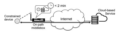
**Figure 4.1** Network scenario with an on-path middlebox that employs a soft-state approach for maintaining information about active connections. The arrow indicates periodic keep-alive messages sent by the communication end-points to keep the connection open.
