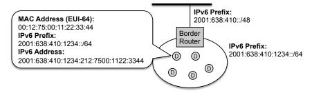
**Figure 2.5** Stateless address autoconfiguration for constrained devices (D) with IPv6. The border router disseminates the IPv6 prefix inside the constrained node network. The constrained devices then complement this prefix to an IPv6 address, e.g., based on their MAC address.
