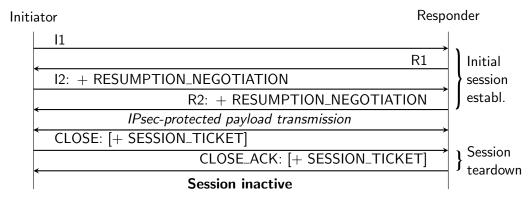
**Figure 4.2** Initial HIP DEX connection establishment with session resumption type negotiation. The session state can be offloaded during the connection teardown. Brackets denote optional parameters that are included depending on the actual session resumption type.
