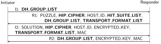
**Figure 4.26** Detailed sequence diagram of the HIP DEX handshake. HIP signaling parameters that are marked bold contain negotiation information that can be compressed. The remaining signaling parameters mainly contain random data with a low compression potential.
