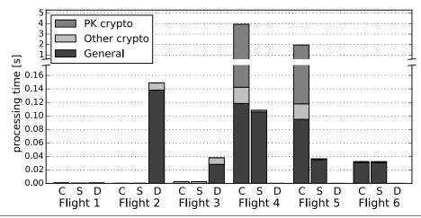
**Figure 5.13** Client-side computation overhead of the certificate-based DTLS handshake (C), the symmetric-key-based DTLS handshake (S) and the presented handshake delegation procedure (D) aggregated on a per-flight basis. The handshake delegation procedure causes a low computation overhead that is comparable to a symmetric-key-based DTLS handshake.
