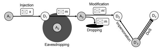
**Figure 3.1** Overview of the network attacks that an adversary can mount in the assumed attacker model. The dark gray circle indicates the radio range of adversary  $A_2$ .  $A_2$  can eavesdrop on network traffic from  $D_1$ .  $A_1$ ,  $A_3$ , and  $D_3'$  can mount injection, eavesdropping, dropping, modification, impersonation, and DoS attacks against the constrained devices  $D_j$ .
