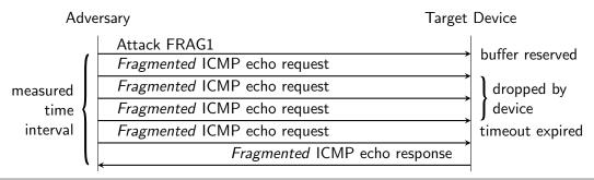
**Figure 6.6** Probing procedure for the continuous timing-based buffer reservation attack. Eve first sends an attack FRAG1 to reserve the reassembly buffer at the target device. She then sends a sequence of fragmented ICMP echo requests that trigger a response from the target device. By measuring the time between sending the FRAG1 and receiving the first ICMP echo response, Eve can estimate the time interval required for the buffer reservation attack.
