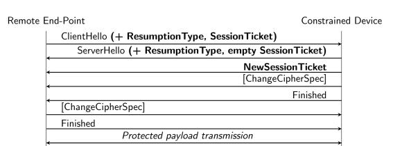
**Figure 5.6** Protocol handshake between the constrained device and the remote end-point in case the remote end-points triggers the session resumption handshake during our delegation procedure. Session resumption-related information is marked bold. Brackets denote protocol extensions. The NewSessionTicket message allows for repeat session resumption handshakes.
