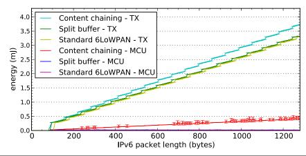
**Figure 6.21** Energy estimation for the computations (MCU) and transmissions (TX) resulting from our presented defense mechanisms on a sending node. The estimated power consumption of the standard 6LoWPAN fragmentation mechanism is given as a baseline. The content-chaining scheme causes non-negligible energy overheads, whereas the split buffer approach exhibits comparable results to the standard 6LoWPAN fragmentation mechanism.
