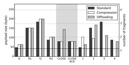
**Figure 4.20** Message size for two subsequent handshakes with an intermediate connection teardown (marked with a gray background) for the *standard* HIP DEX protocol and for session resumption with state *compression* as well as with Initiator-side state-*offloading*. The continuous line indicates the 6LoWPAN fragmentation threshold in our evaluation setup. The dashed lines then indicate the maximum payload size of the individual 6LoWPAN fragments.
