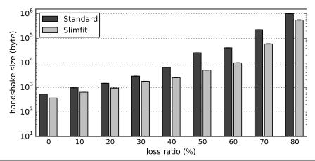
**Figure 4.32** Transmission overhead of the standard *HIP DEX* and the *Slimfit*-compressed connection establishment handshake for different loss probabilities. The error bars depict the 99% confidence intervals. Note the logarithmic scale of the y-axis. The Slimfit-compressed handshake consistently has a lower transmission overhead than standard HIP DEX.
