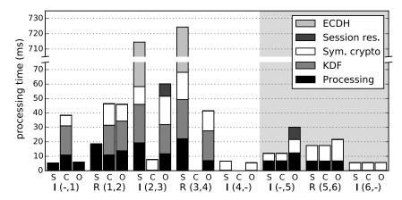
**Figure 4.19** Processing time of the handshake and the connection teardown for the standard HIP DEX protocol (S), session resumption with state compression (C) and session resumption with Initiator-side state-offloading (O) for the Initiator (I) and the Responder (R). The numbers in brackets denote processing of the i-th and generation of the (i+1)-th handshake message.
