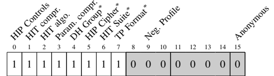
Fig. 5. The compression bits set in the HIP Controls field indicate a HIP DEX packet with maximum Slimfit compression. Negotiation parameter compression flags are marked with an asterisk. Omitted content is highlighted gray. Bits 11 to 14 remain unused.
