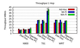
Figure 4: TCP throughput of STANs to different RONs. MA-Fi consistently offers throughput comparable to Wi-Fi and mostly better than ad-hoc mode, except for a few outliers in which MA-Fi performs worse than ad-hoc mode or even better than Wi-Fi.
