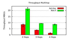
Figure 5: TCP throughput comparison over multiple hops between MA-Fi and ad-hoc mode. In both cases, throughput decreases over multiple hops, however, MA-Fi outperforms ad-hoc mode transmissions over every hop-count.
