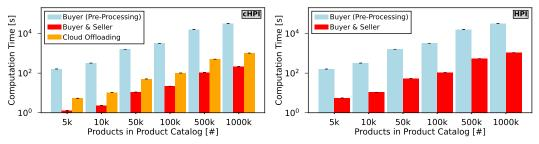
Fig. 11. cHPI (left) reduces the seller's workload by one order of magnitude in comparison to the purely local HPI protocol (right). Thereby, it is a adequate candidate in settings with resource-constrained sellers.
