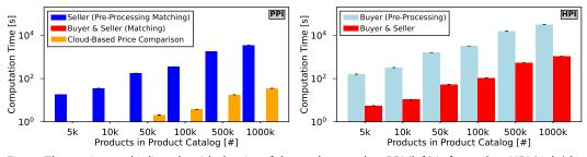
Fig. 6. The runtime scales linearly with the size of the product catalog. PPI (left) is faster than HPI (right) by one order of magnitude. While PPI allows for seller pre-processing, HPI enables buyer pre-processing.
