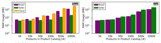
Fig. 12. cHPI (left) significantly reduces the seller's local RAM usage when compared to HPI (right) by utilizing the cloud. Therefore, the virtually unlimited resources in the cloud easily allow for parallel executions.
