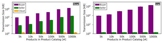
Fig. 13. In contrast to HPI (right), the seller offloads the PHE-based computation to the cloud when using cHPI (left). Thus, companies need to consider the trade-off between computational and network load.
