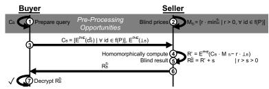
Fig. 5. In HPI, the buyer can pre-encrypt the query using PHE. Subsequently, the seller homomorphically computes a blinded result and returns it to the buyer for decryption, indicating the inquiry's outcome.
