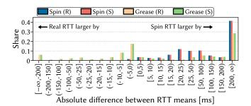
Figure 3: Histogram of abs. difference between means of spin bit and QUIC estimate for all connections.
