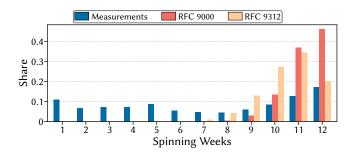
Figure 2: Histogram showing the number of weeks in which the selected domains had the spin bit enabled. RFC values are computed using probability theory and reflect theoretical behavior when the spin bit is disabled in one in eight (RFC 9312) / 16 (RFC 9000) connections.
