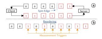
Figure 1: (a): The client of a connection always *flips* the spin bit; the server *reflects* it. (b): Reordering near the spin edges can cause faulty measurements.
