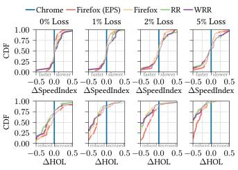
Fig. 6. Impact of Loss on SI and HOL for 2 Mbps Bandwidth and 100 ms RTT
