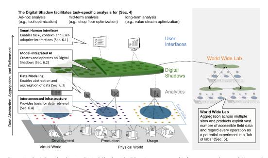
Fig. 2. In the IoP, task-adaptive Digital Shadows build on interconnected infrastructure, data modeling, and model-integrated AI to provide smart interfaces that make the right data actionable at the right time during development, production, and usage. Integration across different production facilities and locations leads to the WWL.
