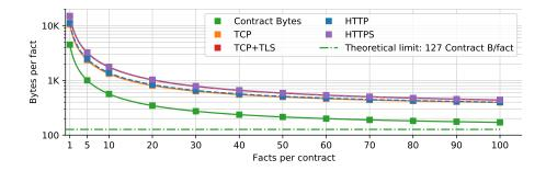
**Fig. 3.** Contract bytes and communication bytes per fact, by the number of facts in one contract. Dataset 1 from Table 1 was used. Communication bytes are split up by handshake mode, i.e., HTTP enabled/disabled, and TLS enabled/disabled. Compared to a per-contract plot, this representation provides better interpretability when comparing the system to other approaches, as contracts are an unknown concept in other work.
