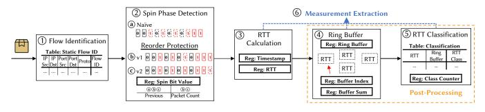
Figure 2: A five-step spin bit tracking pipeline. After an initial flow identification (1) and a spin phase detection (2), our pipeline calculates the current RTT (3). It further keeps track of the last N measurements in a ring buffer (4) and can classify the current RTT based on those last measurements ( $\overline{5}$ ).
