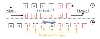
Figure 1: (a): The client of a connection always *flips* the spin bit; the server *reflects* it. (b): Reordering near the spin signal flanks can cause faulty measurements.
