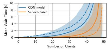
Fig. 6: Mean wait times for CDN and service-based access model with increasing number of clients. Solid lines are simulated results, with shaded areas as standard deviation. Dashed lines are analytical results.
