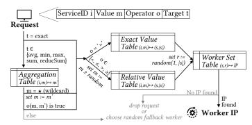
Fig. 4: Depending on the value, operator and comparison target in a request, the service scheduling unit uses different sequences of table lookups, comparisons and lookup value rewrites. A final semi-random lookup in the worker set table yields the IP of a worker able to satisfy the request.
