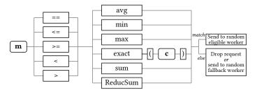
Fig. 2: Constraint model for selecting service instances. Client demands (m, left) are matched against worker supply (right).
