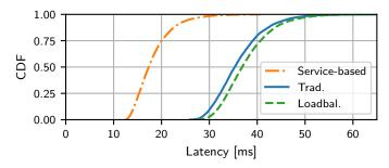
Fig. 5: Expected gains for network latency. Simulation results show that service-based forwarding can significantly cut time to first byte retrieval latencies.
