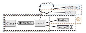
Fig. 1: Testbed topology with testbed and online components. Scenario (a) (testbed-only), Scenario (b) (testbed & Internet), Scenario (c) (Internet-only).
