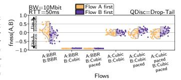
Fig. 2: Results from Scenario (a) for 10 Mbps, 50 ms and a buffer of 0.5×BDP for different CC algorithm combinations.
