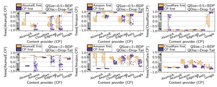
Fig. 5: AkamaiE, Amazon, and Cloudflare competing against the other content providers in the 10 Mbps, 50 ms setting. Amazon performs similar to Edgecast and Fastly, Cloudflare is similar to Google. Top row shows  $0.5 \times BDP$ , bottom row  $2 \times BDP$ .
