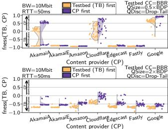
Fig. 4: A BBR flow originating from our testbed competes with the content providers for traffic using a small buffer (top) and a large buffer (bottom).
