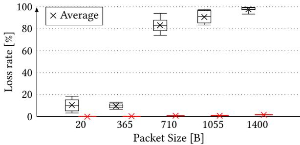
Figure 6. Measurement of PRRT for different packet sizes, receive window of 480 μs, target delay of 1000 μs (black) and 3250 μs (red)
