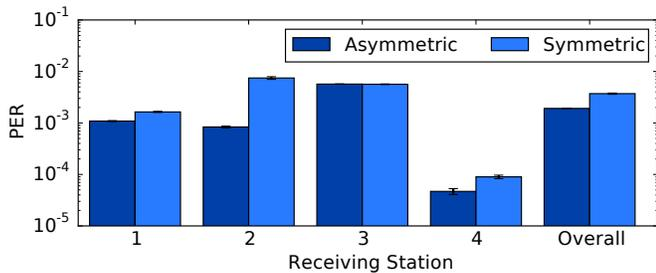
Fig. 9. PER of the relaying process when collecting asymmetric CSI compared to symmetric CSI.
