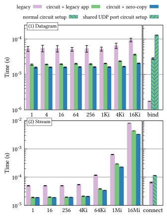
Figure 4: RTT for different response sizes (byte) and the response time of the bind and connect operation.
