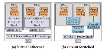
Figure 2: Comparison of the virtual Ethernet approach to our circuit-switched VM networks aprroach.
