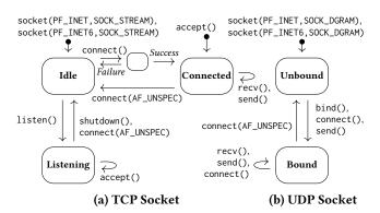
Figure 1: Most important socket states and functions.
