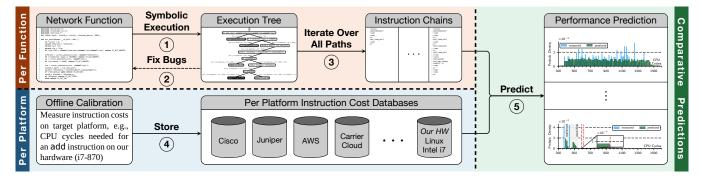
Figure 1: SymPerf architectural overview and Network Function performance prediction workflow.
