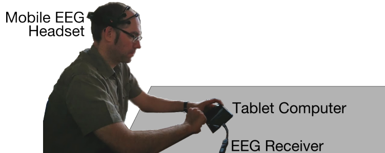
Figure 1. Experiment set-up with a Study Participant. Note, the equipment is small, mobile and easy to transport.
