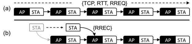
Fig. 3. Topologies to evaluate (a) throughput, round trip time and route request delay and (b) route recovery delay in case of STAN mobility.
