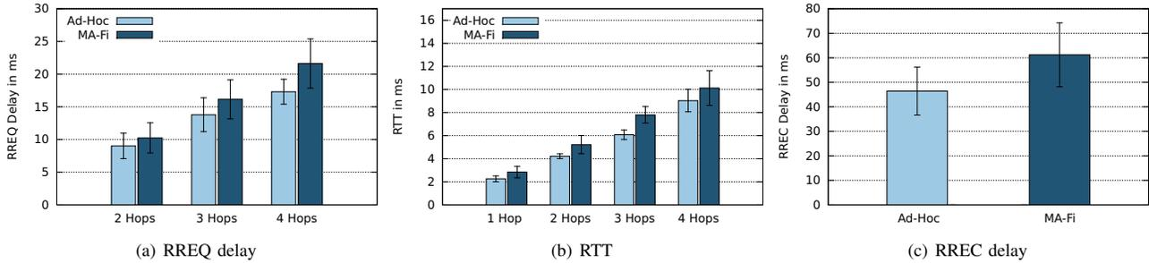
Fig. 5. Route establishment, round trip time, and route recovery performance of MA-Fi over increasing hop counts, in comparison to the 802.11 ad-hoc mode.
