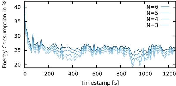
Fig. 8. Cumulative network-wide energy consumption of duty cycled RONS and associated STANs relative to ad-hoc mode consumption.
