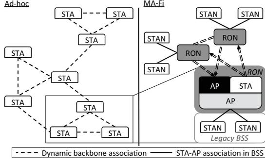
Fig. 1. Topological illustration of an ad-hoc mode network (left) and an equivalent MA-Fi network (right). RONs establish a meshed backbone network that connects the legacy networks provided at each RONs .
