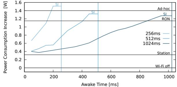
Fig. 7. Energy savings, compared to 802.11, follow a trade-off between the switching interval (SI) of the Wi-Fi card and 802.11 driver, the response time of the network and the awake time in each duty cycle interval (256/512/1024 ms).
