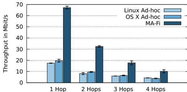
Fig. 4. Multi-hop TCP throughput of MA-Fi in comparison to ad-hoc mode.
