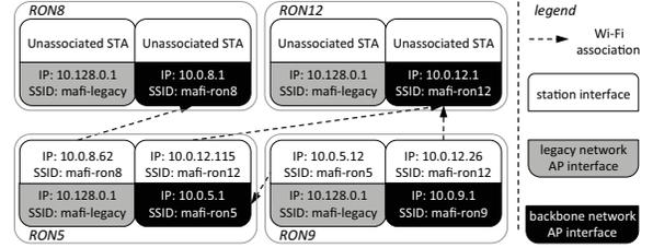
Fig. 2. RONs operate multiple virtual interfaces in station (STA) or access point (AP) mode. Identical AP interfaces at RONs span a continuous legacy network, while RONs connect to backbone networks of other RONs as stations.
