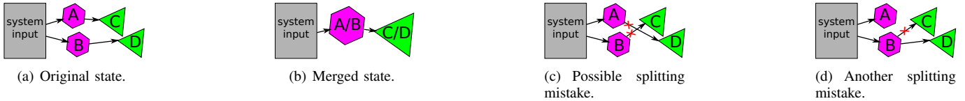
Fig. 3. Possible problems when not providing a reasonable history of the connections and splitting multiple modules.
