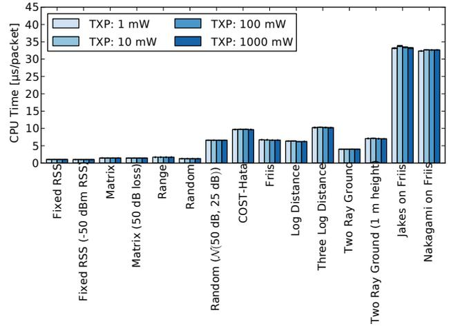
(b) Computational effort to compute the receive signal strength of one packet at all potential receivers by means of different propagation models
