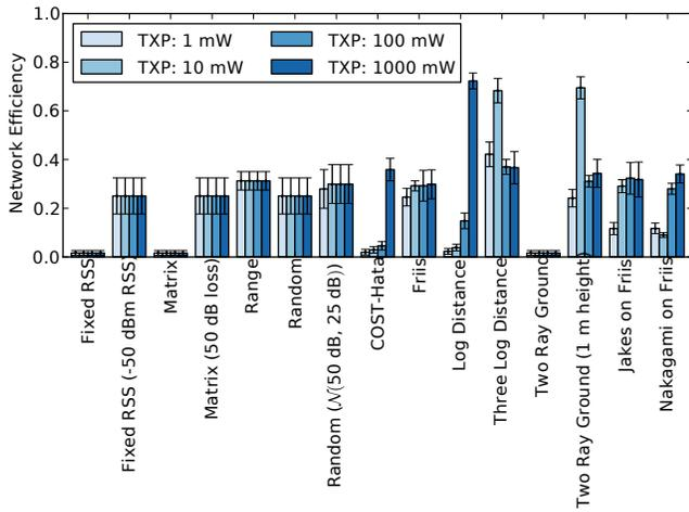
(a) Network efficiency (number of successfully received packets at destinations over the number of packets transmitted)
