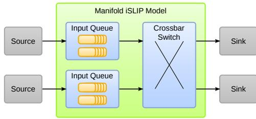
Fig. 1. The *iSLIP* Model for a  $2 \times 2$  Router.
