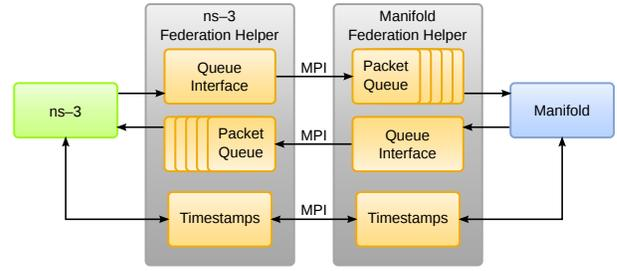
Fig. 3. The MPI based scheme utilizes two federation helpers communicating via MPI messages for packet transmission and time synchronization.
