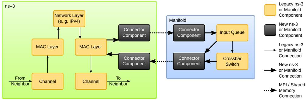
Fig. 4. We added 2 new components to each model for packet exchange, and modify the *ns-3* MAC layer slightly.
