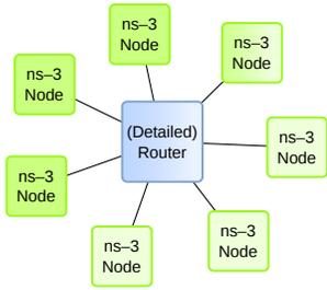
Fig. 5. The Topology of our Evaluation for an Exemplary 7 Node Network
