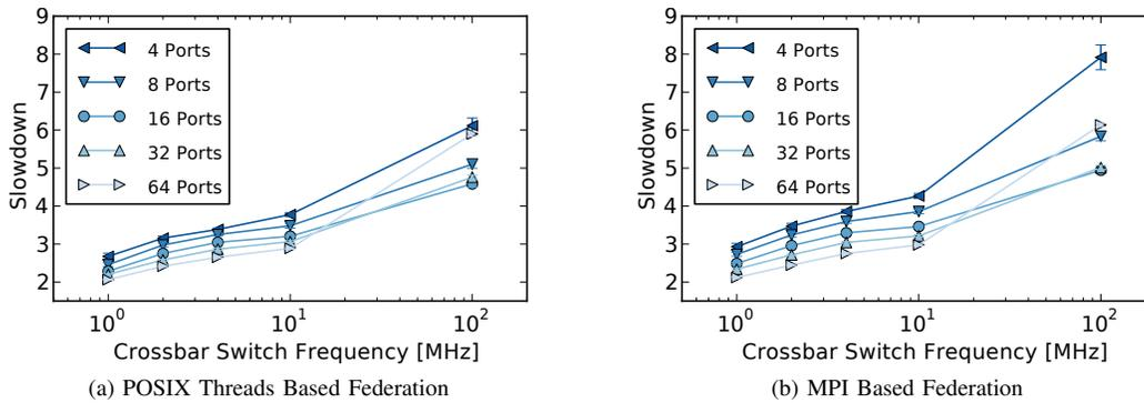
Fig. 9. Overall Slowdown in Simulation Performance
