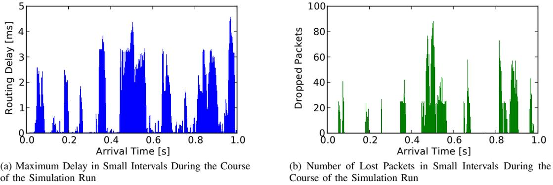
Fig. 8. Delay and Packet Loss at an Input-queued Router Computing 220,000 Matchings per Second
