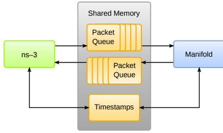
Fig. 2. The thread based scheme utilizes the shared memory for packet transmission and time synchronization.
