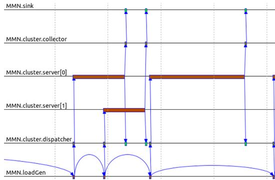
**Figure 1:** Screenshot showing the duration of events illustrated by the length of the “event-block” while event complexities are color-coded. Note the difference in complexity: Events on the server and load-Gen modules are more complex (darker) than events on the dispatcher or sink (lighter).
