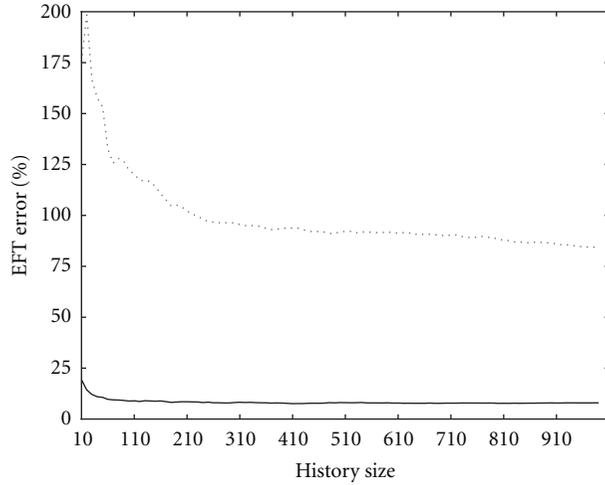
(a) Settling Time:  $MAC_3$  shows a faster convergence towards its base value over the history size and achieves a smaller estimation error (7%) than  $\beta$ . Based on data of the Mirage testbed
