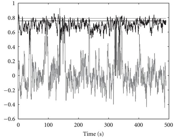
(b)  $MAC_3$  generates more accurate and more stable results over time than  $\beta$ . The straight lines show the base values of both metrics over the entire transmission trace
