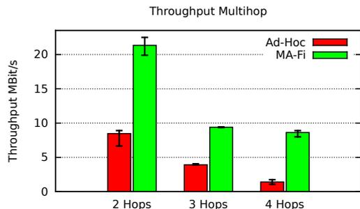
**Figure 5: TCP throughput comparison over multiple hops between MA-Fi and ad-hoc mode. In both cases, throughput decreases over multiple hops, however, MA-Fi outperforms ad-hoc mode transmissions over every hop-count.**
