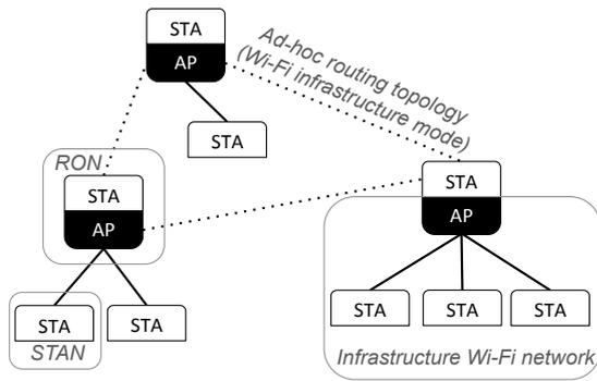
**Figure 1: Nodes provide autonomous 802.11 infrastructure mode networks to stations. Additionally, nodes maintain associations to networks provided by other nodes to achieve interconnectivity and multi-hop communication.**
