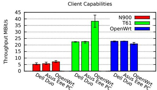
**Figure 2: TCP throughput of two netbook devices (Asus Eee PC, Dell Duo) serving as RONs for different STAN types. As a reference, results of a WLAN router (OpenWrt) are shown.**
