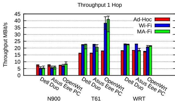
**Figure 4: TCP throughput of STANs to different RONs. MA-Fi consistently offers throughput comparable to Wi-Fi and mostly better than ad-hoc mode, except for a few outliers in which MA-Fi performs worse than ad-hoc mode or even better than Wi-Fi.**
