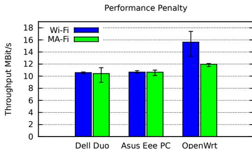
**Figure 3: Throughput between two STANs connected to the same node in Wi-Fi and in MA-Fi. Operating an additional STA interface in MA-Fi reduces throughput, but still allows for good throughput between STANs.**
