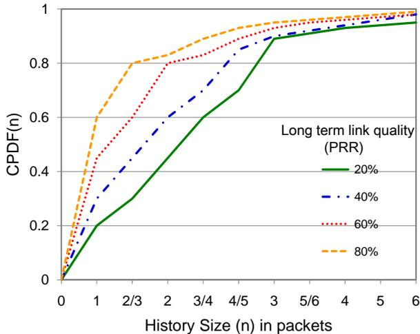
Fig. 1. Measuring the impact of recent transmission success over a link on the next transmission over that link. A label of  $k/n$  stands for  $k$  successes during the last  $n$  transmissions, and  $n$  is a shorthand for  $n/n$ .  $CPDF(n)$  is the probability that the next transmission is successful.
