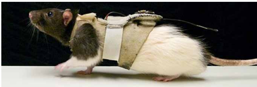
Fig. 1. An example of a laboratory rat wearing a mica2dot sensor node on a removable harness
